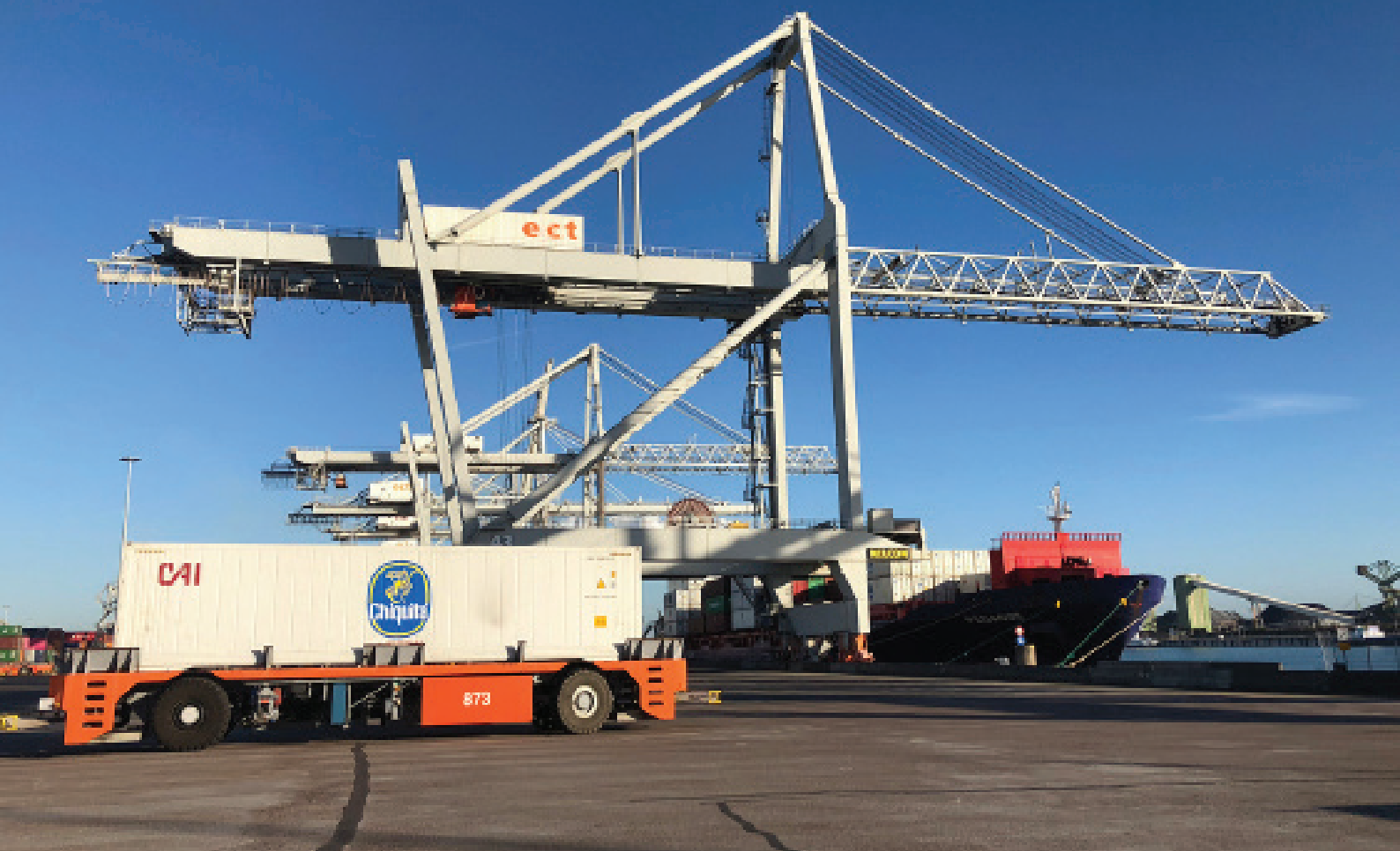
ECT container cranes and Automated Guided Vehicle-AGV system. (© Leon Willems, 2020; Source: Port of Rotterdam Authority).
