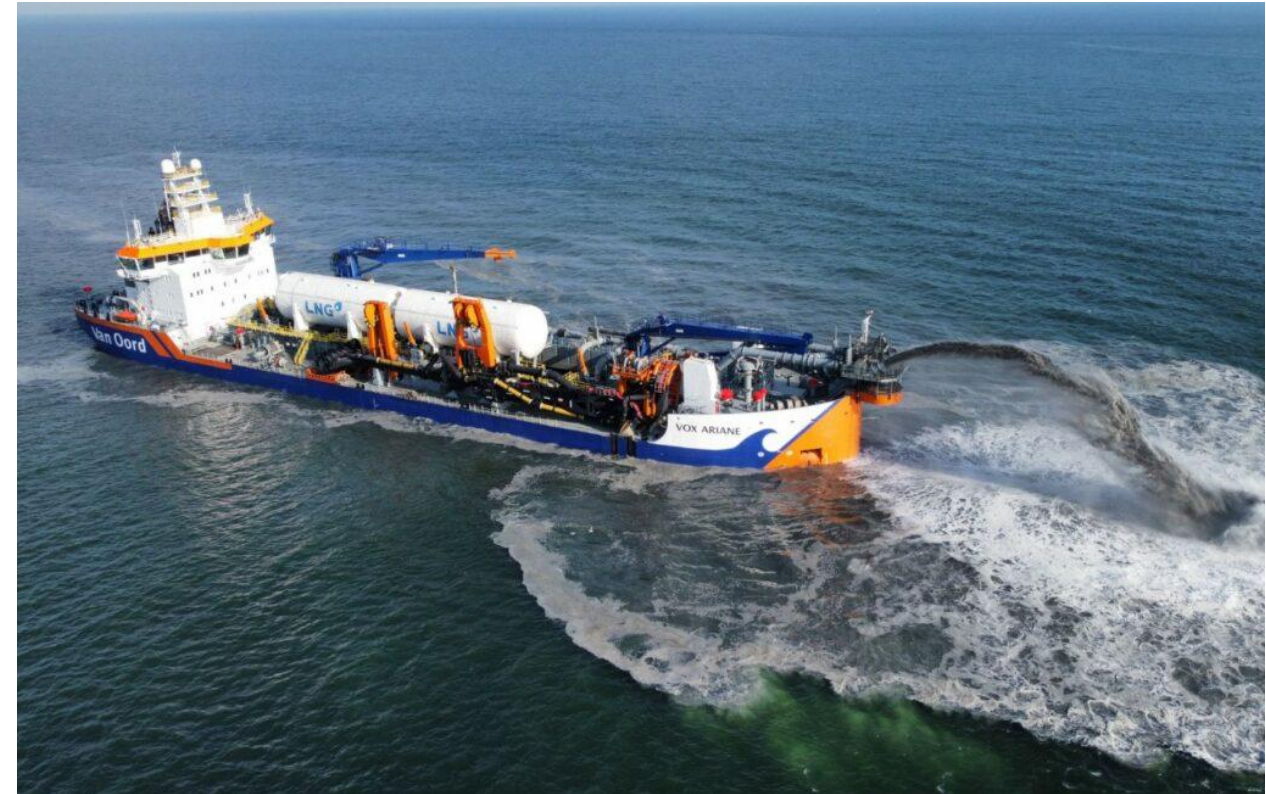
Vox Ariane: Van Oord's first TSHD equipped with an LNG fuel system
