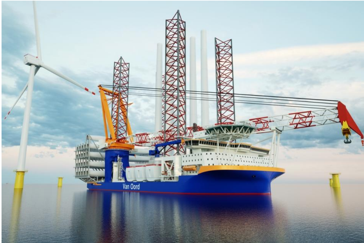
Boreas: A new methanol electric installation vessel for offshore wind
